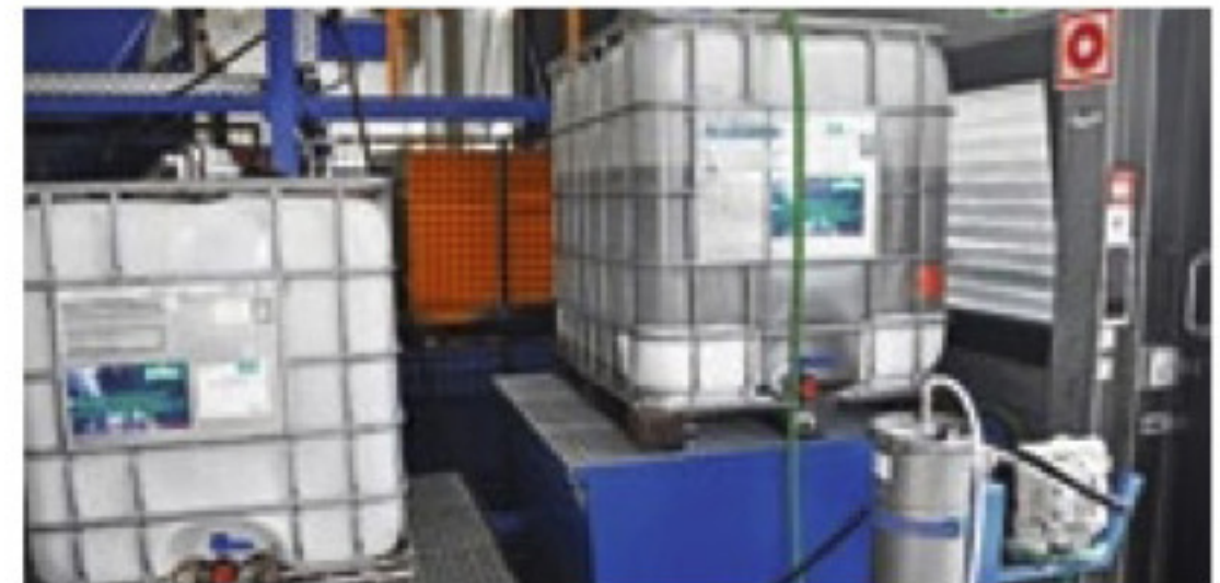
The recovered cutting oil is purified using filtration equipment, then returned to the machine tools along with a portion of fresh oil.
