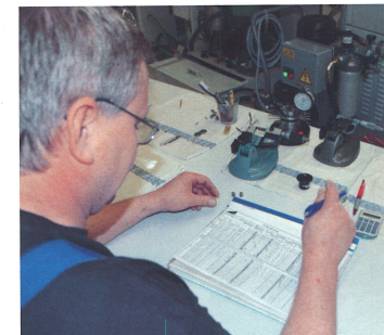
The machine operator stays informed by taking regular measurements and keeping a measurement log.
