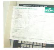
The cutting data control sheet developed by MOTOREX is used to record and easily compare all relevant parameters.
