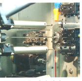
ORTHO NF-X allows flawless boring (to a depth of 108 mm) at only 40 bars of cutting oil pressure.
